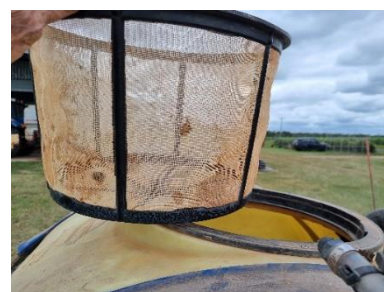
Photo 3 – Screen in tank
