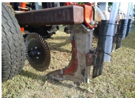
Photo 3 – Brew injection & seeder
