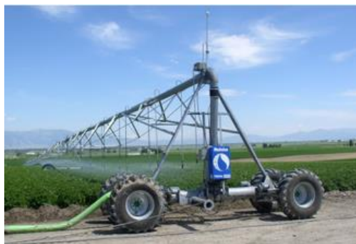
Photo 5 – Low pressure irrigator
