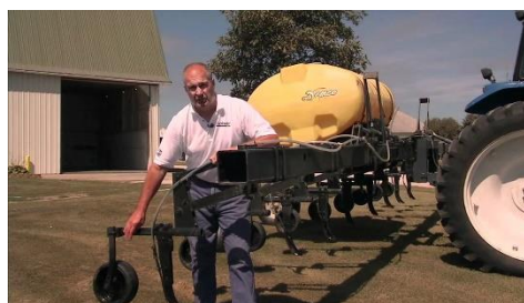
Photo 1 – Rear mounted tank
