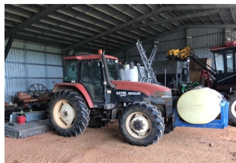
Photo 2 – Front mounted tank
