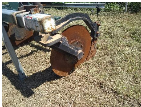
Photo 4 – Brew injection behind coulter
