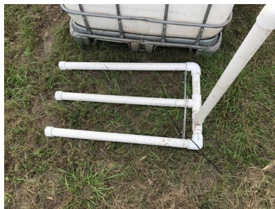
Photo 2 – Air spreader pipes
